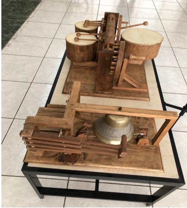
Above models are of automated drums and a bell ringer with actual keys to press
