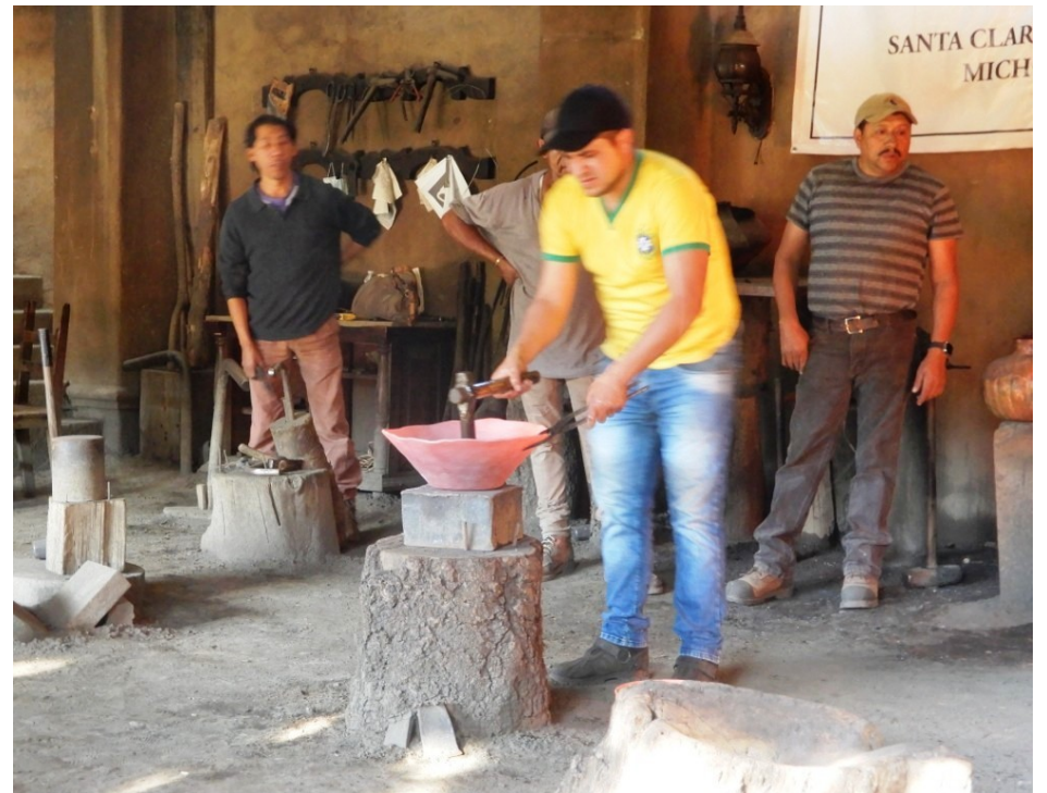
A demonstration in a workshop took red hot copper from a forge like a blacksmith's to show how it could be shaped by hammer while the copper was still hot.
