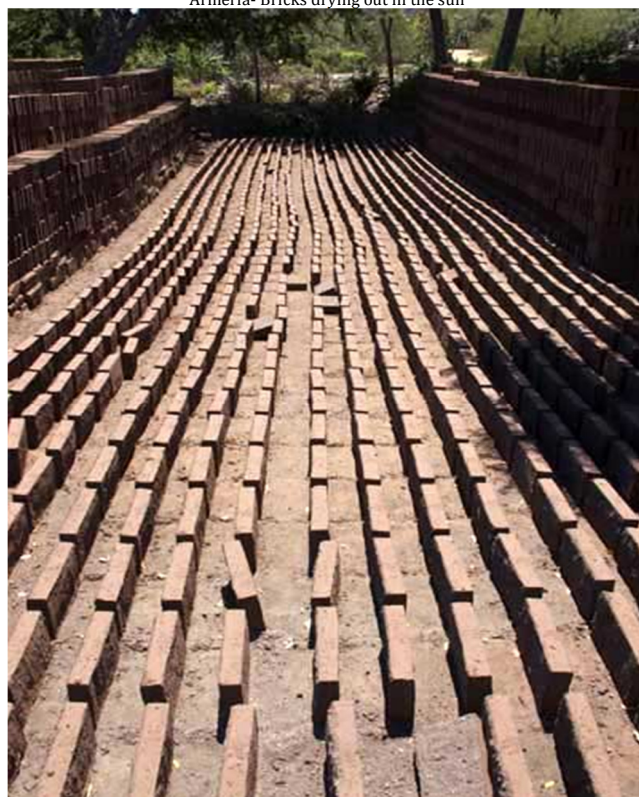
Bricks on the ground are repeatedly turned on edge
